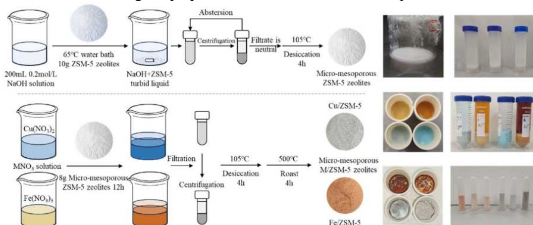
Figure 4: Synthesis of micro-mesoporous ZSM-5 and M/ZSM-5 molecular sieves
