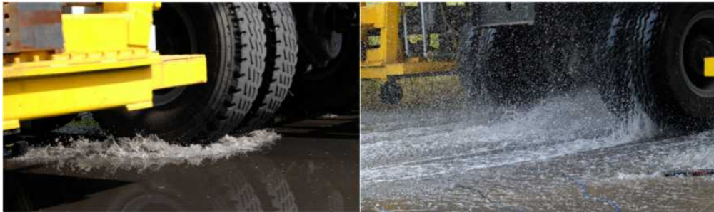
Dynamic Hydraulic scouring induced by a moving vehicle
