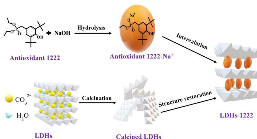
Figure 1 Schematic diagram of synthesis of LDHs-1222
