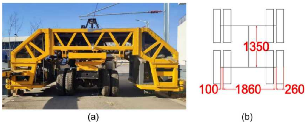
Figure 1.2 (a) Front view of the Loading axles; (b) Top view and the size of the frame (unit: mm)
