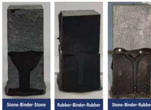
(a) Three interfaces in the mixture
